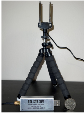
Fig. 2. RTL-SDR RTL2832U DVB-T tuner dongle and antenna used to passively receive the spectrum.
